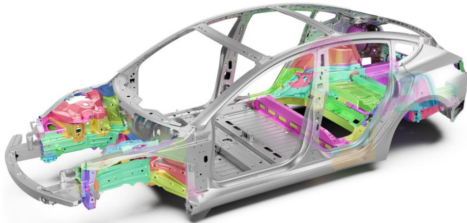
Model 3 body structure 171 pieces of metal highlighted
