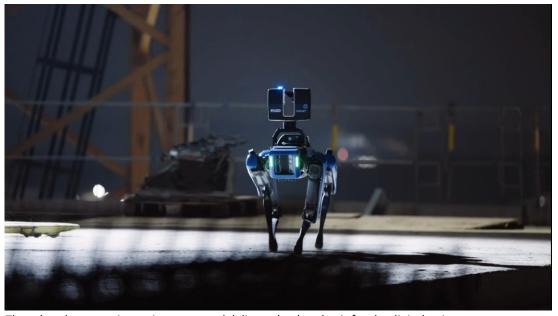
The robot dog scans its environment and delivers the data basis for the digital twin. © Behind the Mask
